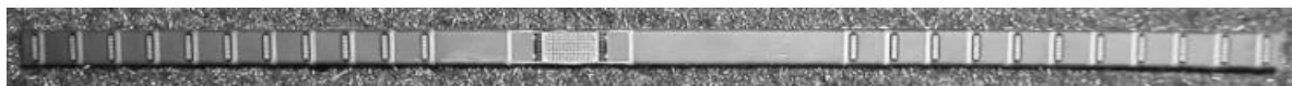
Figure 6. The eight layer flexible circuit used to build the 5 MHz laparoscopic transducer.
