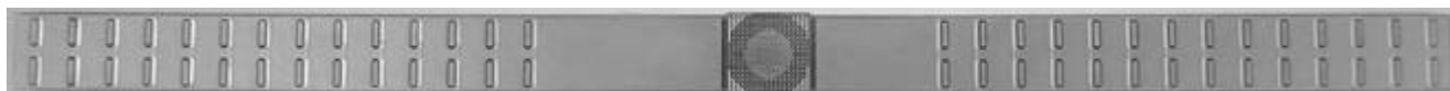
Figure 7. The ten layer flexible circuit used to build the 7 MHz laparoscopic transducer.
