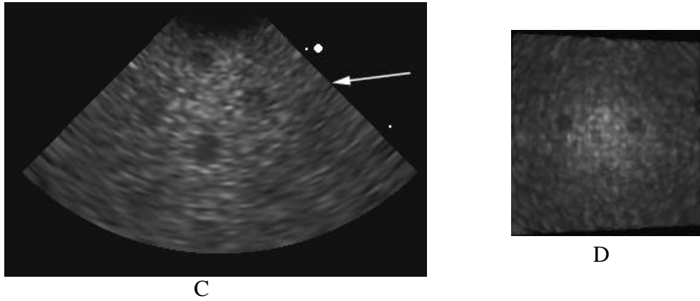
Figure 12. Images from the RMI spherical lesion phantom. Figure 12A is a 3 cm deep 90° B-scan, and fig. 12B is the corresponding real time C-scan made at the plane indicated by the arrow. Both images were made with the 5 MHz laparoscopic transducer. Figures 12C and 12D show the same phantom using the 7 MHz laparoscopic transducer. The higher frequency and larger aperture of the 7 MHz transducer result in an improved image with better boarder detection of the lesions and a finer speckle pattern.
